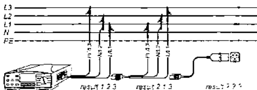
Fig. 35. Connection of Universal test cable and Three phase cable
