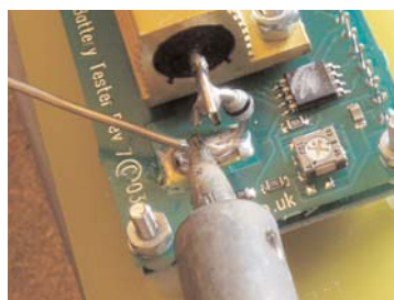
Step 8 Solder in Diode (black band to resistor).
