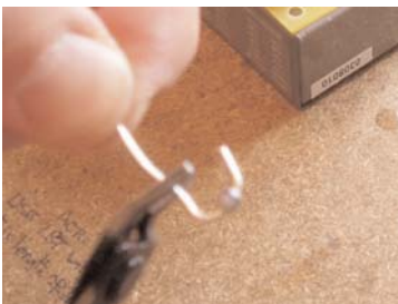
Step 7 Make link with supplied Diode.
